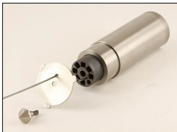
Figure A25. An empty ICSA MAX phase irradiation capsule (HT) before irradiation.
