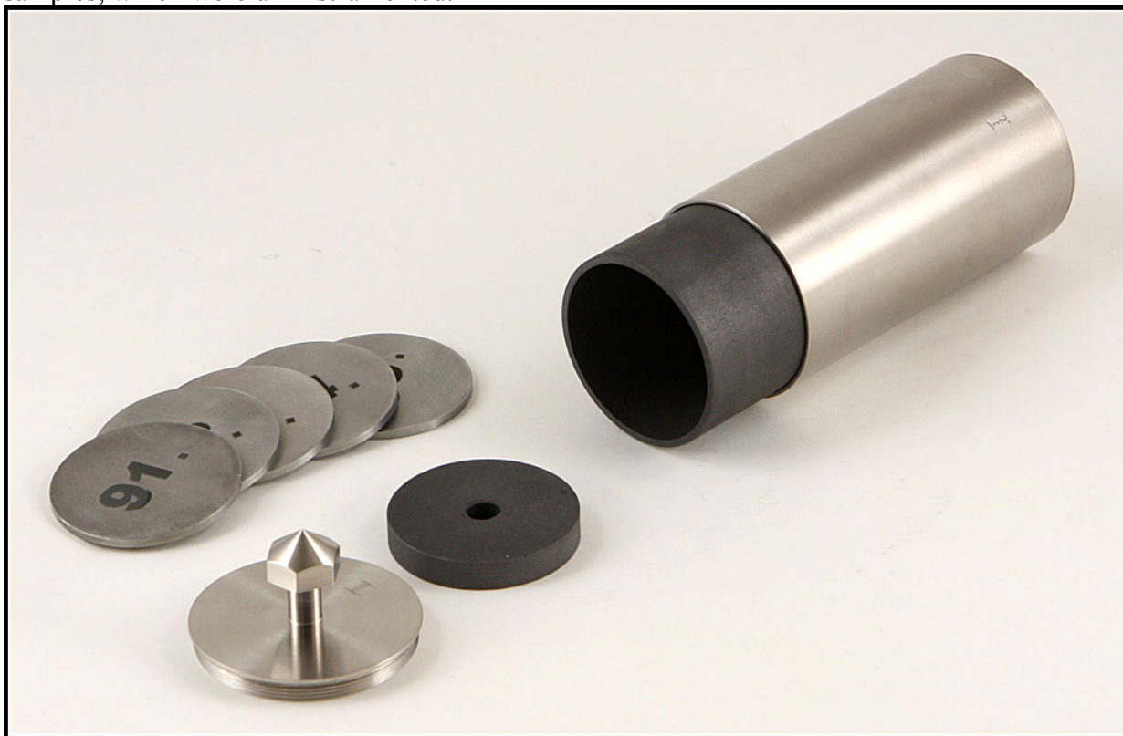
Figure A23. ICSA capsule with graphite spacer, liner, and Mo metal disks.
