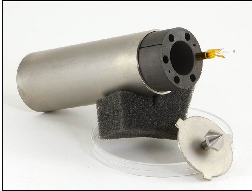
Figure A28. Titanium capsule and graphite holder with one fiber optic sensor loaded for ICSEA irradiation.
