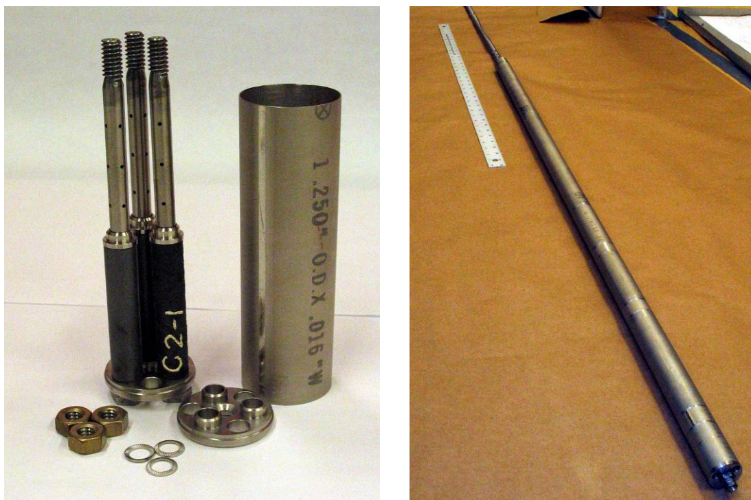
Figure A3. Photographs of a sample module during assembly and the fully assembled sample stack before insertion into the autoclave.
